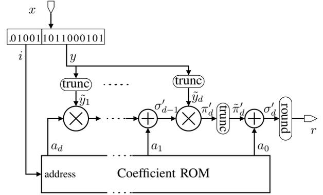
Figure 3. The function evaluation architecture
