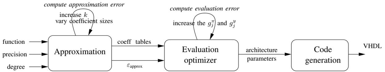
Figure 1. Automated implementation flow
