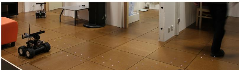
**Fig. 12** Picture of the apartment in the LORIA Lab. The ground is composed of a network of intelligent tiles. Each tile embeds a node that is able to store, compute and display information as well as communicate with neighboring tiles and nearby robots. LED lighting indicates that the tiles have detected the presence of people or robots (see <http://infositu.loria.fr>).
