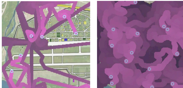
Fig. 2. Base patrolled by a set of UAVs dropping a visit pheromone: initial exploration phase (left) and stabilized phase (right). Brighter color means more pheromone.
