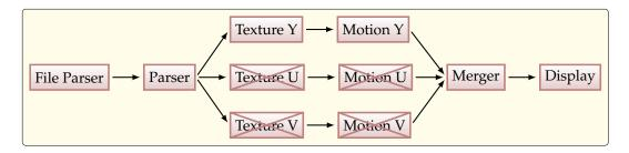
Figure 4: Optional Processes in MPEG 4 part 2 Simple Profile Decoder
