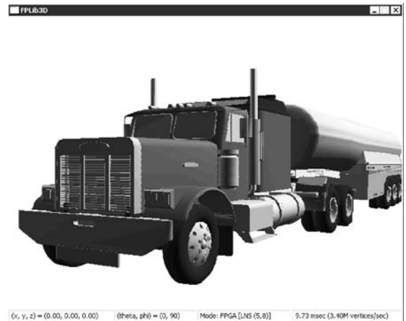
Figure 12. 3D image, using method LNS-O1 and precision (w_E, w_F) = (5, 8) .
